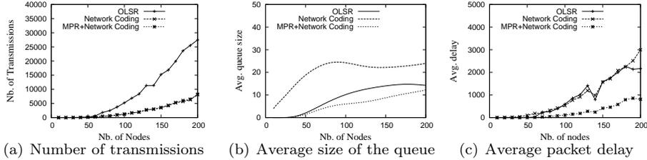
Figure 4: performance comparison of MPR-based coding and OLSR and only-network-coding-based flooding.
